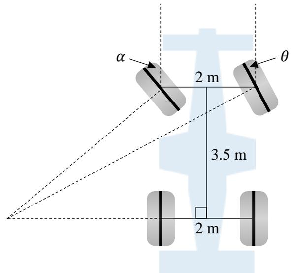
One steering system that will ensure the angle of the inside wheel is closer to the values in the table above is shown below. The front wheels are connected by a beam that is shorter in length than the distance between the wheels. This results in the wheels turning at different angles.
