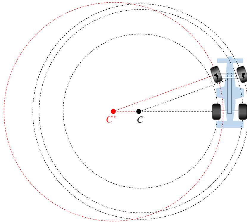
Before we can develop a system, we should determine at which angles the inside-front wheel should turn when the outside-front wheel has turned by specific angles. Suppose the distance between the centres of the front and rear wheels is 3.5 m and the distance between the centres of the left and right wheels is 2 m. Use the diagram below to complete the table.
