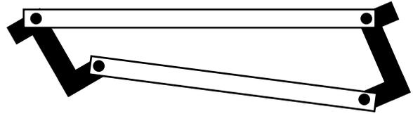
A simplified representation of this system is shown in the diagram below. When the outside wheel is turned by an angle of  $\theta$  the inside wheel turns by an angle of  $\alpha$ . Use the diagram to complete the table.
