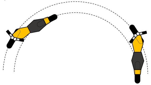
The arcs both have the same centre, but their radii depend on the angle at which the front wheel is turned, and the distance between the centres of the wheels.
