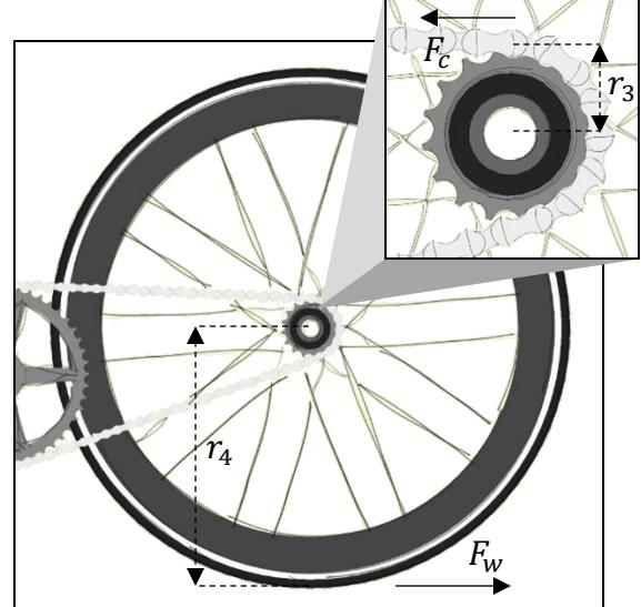
Suppose the radius of the sprocket is  $r_3$ . The chain exerts a force on the sprocket of  $F_c$ .
