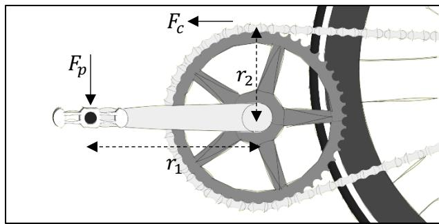
Suppose the length of the crank arm is  $r_1$  and the rider exerts a force on the pedal of  $F_p$ .
